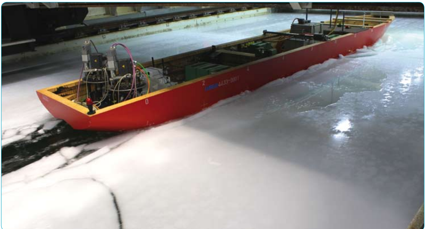
Fig. 5: Model in pressurized zone with transverse crack
