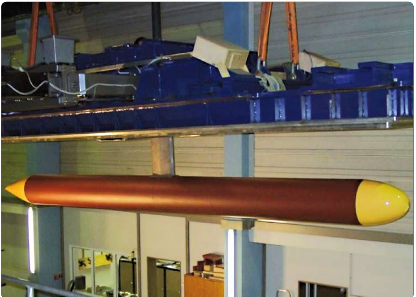
Fig 1: 8 m long axis-symmetric body for laboratory test
