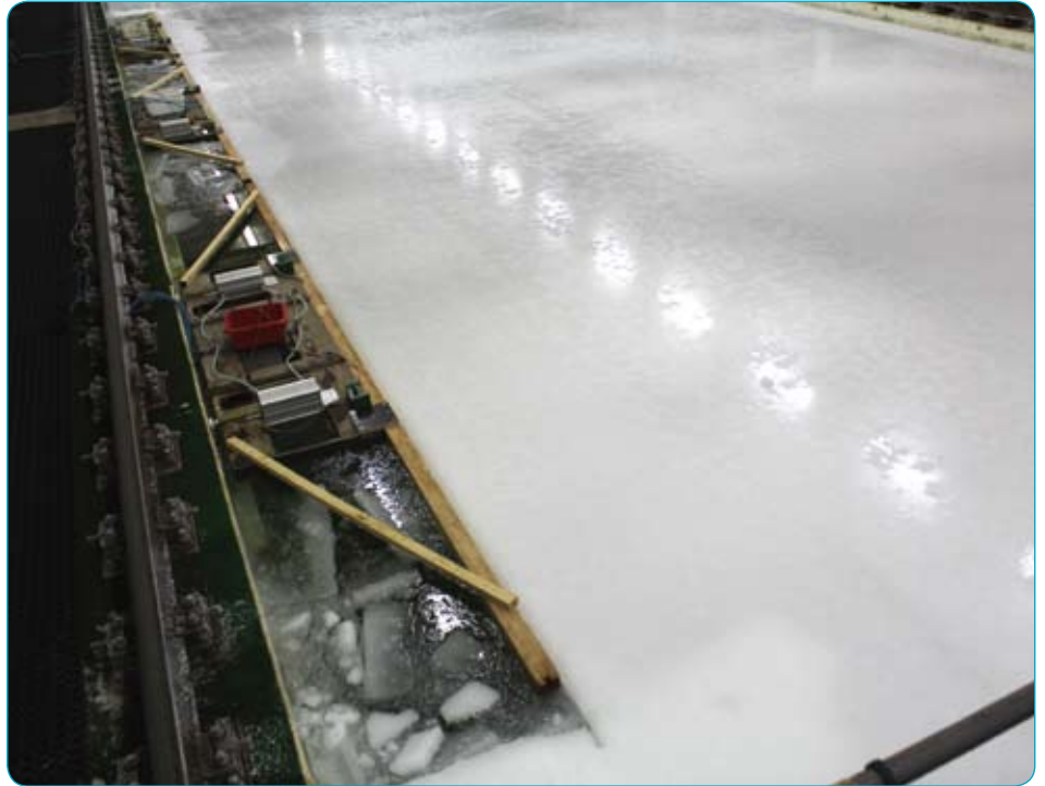
Fig. 4: Installation of side pressure device in ice basin
