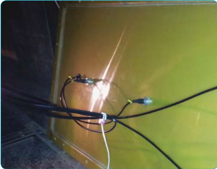
Fig. 3: Window made of GRP sandwich with part of the sensor equipment
