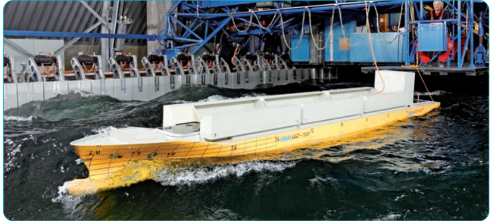
Fig. 4: Container Ship in Severe Stern Quartering Short Crested Seas
