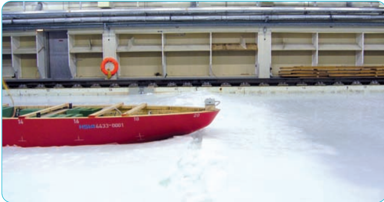
Fig. 2: Ship model breaks through model ice ridge
