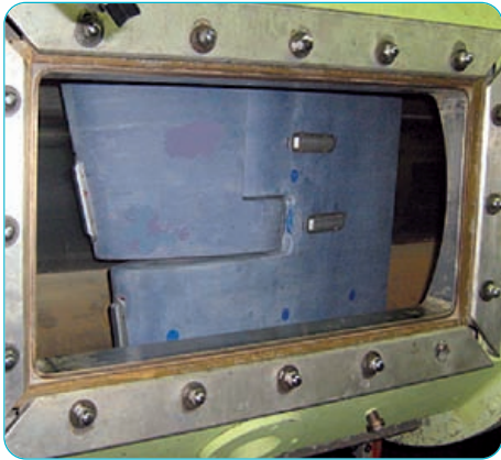
Fig. 2: Large Scale Part Rudder Model
