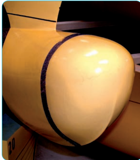
Fig. 1: Pronounced bulbous bow as result of a “single-point” optimisation
