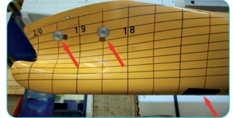
Fig. 2: Slamming Panels in the bow section
