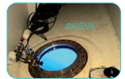
HSVA's Class Approved Observation Window in the Shell
