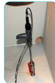
HSVA's Boroskop Looking Through a Tiny Hole in the Shell
