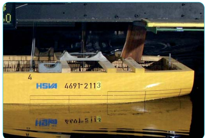
Ship model during the calm water tests
