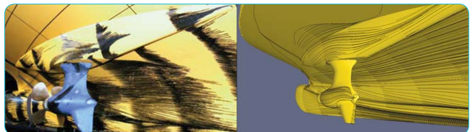
Fig.2: Comparison of wall streamlines obtained from model test and CFD prediction
