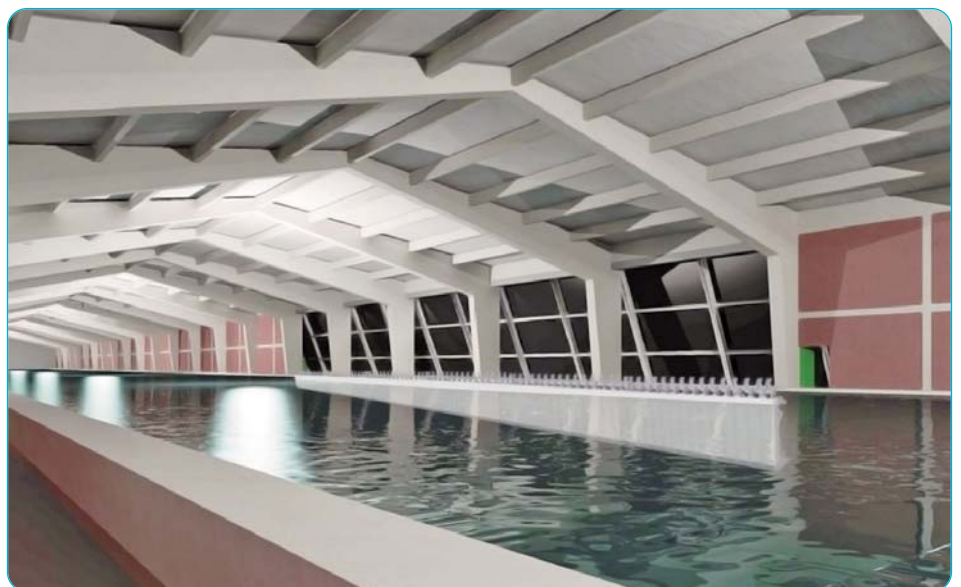
Fig.1: Impression of the new side wave generator in the large towing tank
