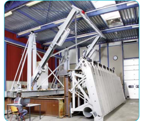
Fig.2: One section of 8m length of the wave generator
