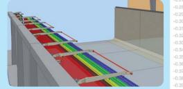
Fig. 3: Wave absorbers on the opposite tank wall
