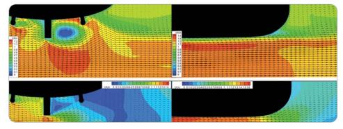
Fig. 3: Velocity distribution of a RANS computation in deep and shallow water
