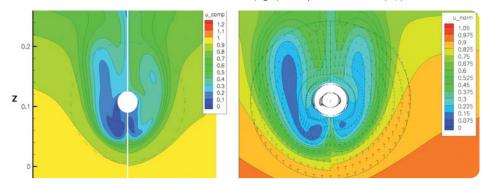
Wake Optimisation:Tanker hull (left), Bulk Carrier (right), each showing the baseline design on the left and the optimised hull on the right.
