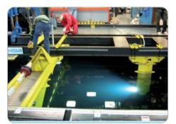
Fig. 4: Towing carriage installation
