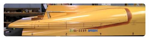
Fig. 2: The model of the 'after conversion' Hammerodde under construction in HSVA's model workshop
