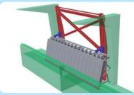
Fig. 2: Stowed side wave generator with hoisting system
