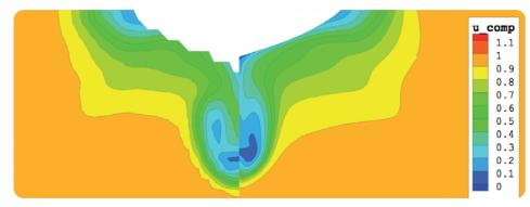
Validation: Tanker Hull: FreSCo Results (right) vs. experimental data (left)
