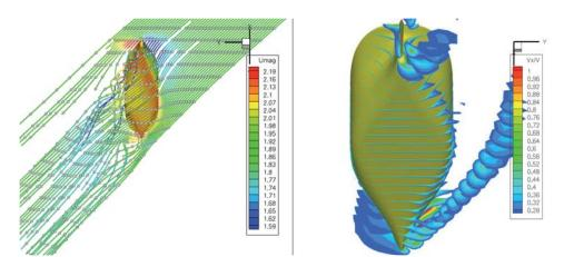
Predicted streamlines and hull pressure distribution (left) and axial flow field velocity (right) for a yaw angle of 30°
