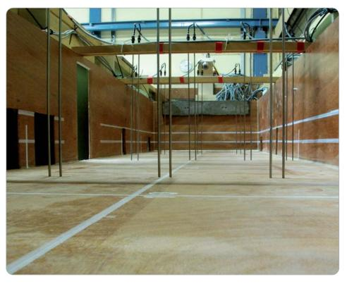
Fig. 2: A view of the vehicle deck during the outfitting of the model. In full scale the deck is about 44 m long. The arrays of the wave probes cross the otherwise open deck. The large black opening on the left side wall is the modeled collision damage by another ship bow.
