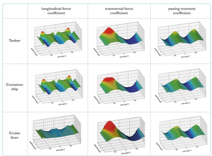
Fig. I: Oblique towing test results in deep and shallow water
