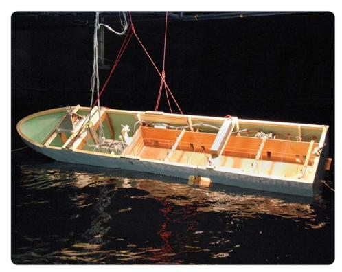
Fig. 4: A ship model at the end of a short damage stability test in irregular seas.
