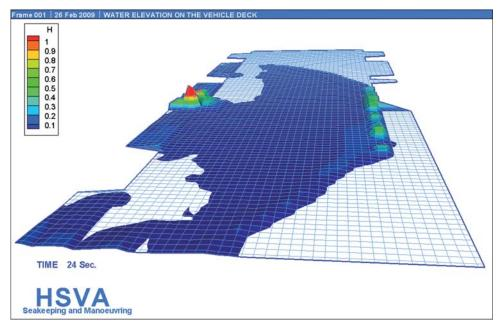
Fig. 3: A snap-shot of the numerically simulated flow on the vehicle deck of the rolling ship in seaway shortly after the simulation started. The color-scale of the water height on the deck is in meters. The side compartments connected to the vehicle deck with door openings are included in the model.
