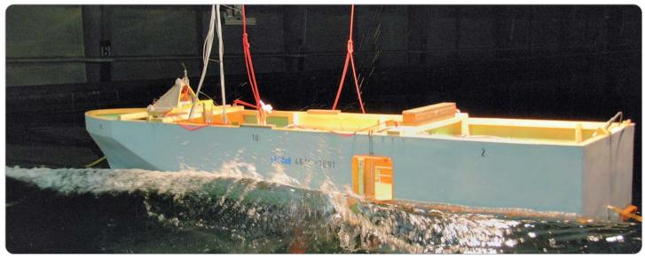
Fig. 1: A ship model in an early phase of a damage stability test in waves in the HSVA towing tank. The photograph shows a breaking wave just before it hits the damaged ship side and pushes considerable amount of water through the damage opening mainly on to the vehicle deck.
