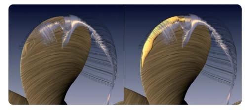
Predicted Tip Vortex roll-up and cavitation pattern (right) for the INSEAN Test Case in VIRTUE
