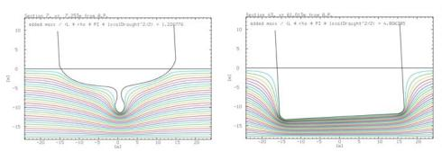
Fig. 4: Simple potential flow in shallow water for a fast estimation of hydrodynamic added masses
