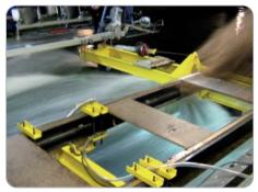
Fig. 5: Tests with a towing speed of 10 m/s
