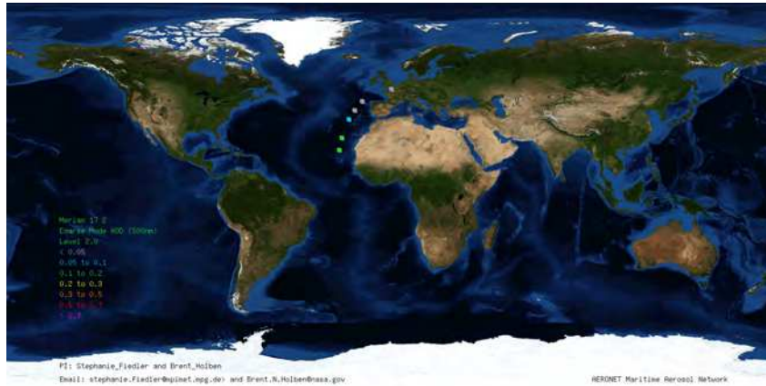
Figure 31: Daily mean coarse-mode aerosol optical depth. Shown are the coarse-mode aerosol optical depth at 500 nm from the level 2 product of the measurements with the sun-photometer MICROTOPS for the AERONET's Maritime Aerosol Network (MAN) of NASA.
