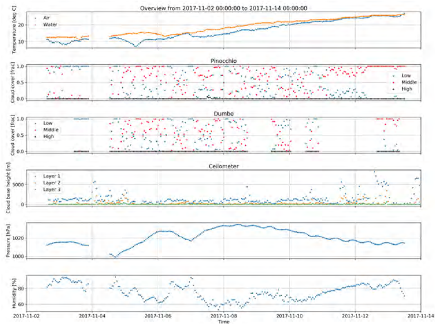
Figure 25: Overview from MCloudS software. Shown are the time series of the preliminary cloud fraction retrievals per height layer from the imagers 'Pinocchio' and 'Dumbo', the backscatter heights indicating the cloud base from the Ceilometer, and measurements from the onboard meteorological instruments of the vessel, i.e., sea and air temperatures, air pressure and relative humidity, for the entire expedition MSM 68/2. All values are hourly means excluding missing data.
