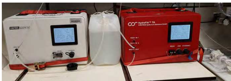
Figure 56: The Contros HydroFIA ® TA set-up in the chemistry lab of the RV Maria S. Merian (Photo: Katharina Seelmann)
