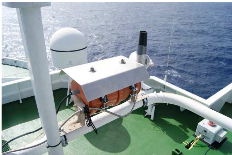
Figure 38: Telescope unit of the MAX-DOAS system mounted aboard MARIA S. MERIAN.
