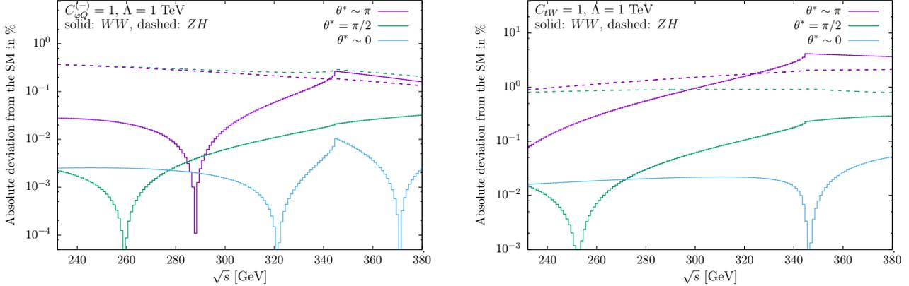
Fig. 3. Center-of-mass energy dependence of  $O_{\varphi Q}^{(-)}$  (left) and  $O_{tW}$  (right) contributions to  $e^+e^- \rightarrow W^+W^-$  (solid) and  $Zh$  (dashed) production in percent of the SM rate, for  $C/\Lambda^2 = 1$  TeV $^{-2}$ . Dependences are shown in absolute values (changes of sign generate the visible dips) for three different scattering angles: 0,  $\pi/2$  and  $\pi$ . For  $e^+e^- \rightarrow Zh$ , the 0 and  $\pi$  curves overlap.
