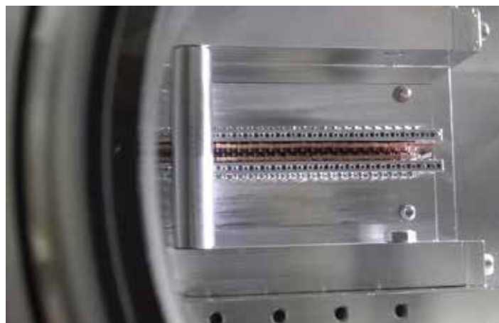
The undulator of LUX in which the fast electrons emit X-ray radiation
