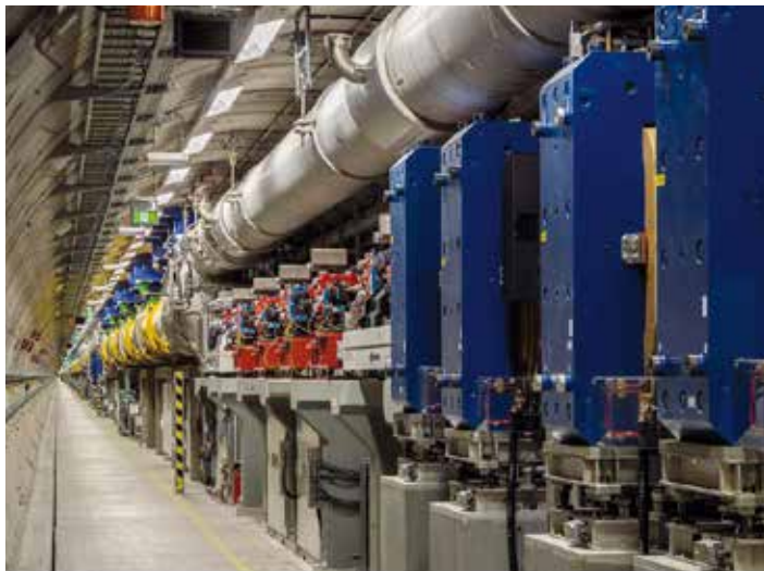
View into the European XFEL accelerator tunnel: Behind a chicane (in front) operating at room temperature, the electrons are guided into the first four superconducting accelerator modules (yellow).
