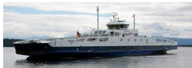
Fjord1's Fannefjord was converted into an LNG battery hybrid in 2016.
