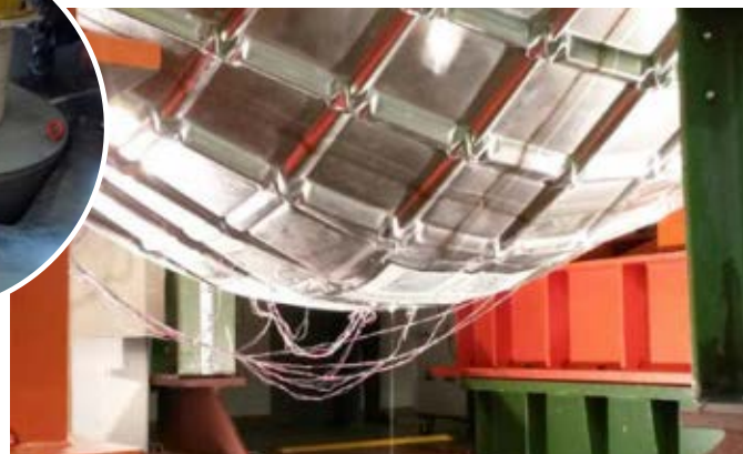
Test rig following the impact of the bulbous bow dummy (left) on the membrane tank mock-up, showing the deformation (right).
