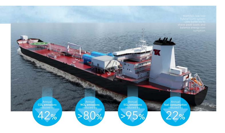
generated and enables more fuel savings through peak load shaving and added overall system redundancy while minimizing the impact of a failure during DP operation.
