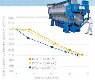
Relative maximum continuous rating in relation to LVOC mass ratio in per cent in LNG mixes.
