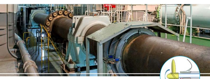
DNV GL has revised the main class rules for single stern tube bearing installations and now offers new optional shaft alignment class notations. Downward bending moment induced during a starboard turn on a single-screw right-handed propeller.
