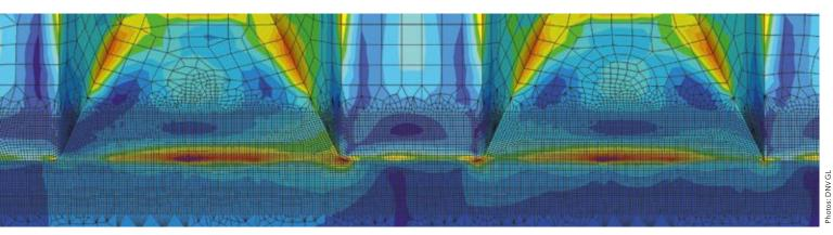
Feasibility study of product/chemical tanker. Maximum surface stresses (for hotspot stress assessment) at lower hinge of transverse bulkhead (see high stress concentration in way of inclined plate corner located close to a diaphragm web plate in lower stool).
