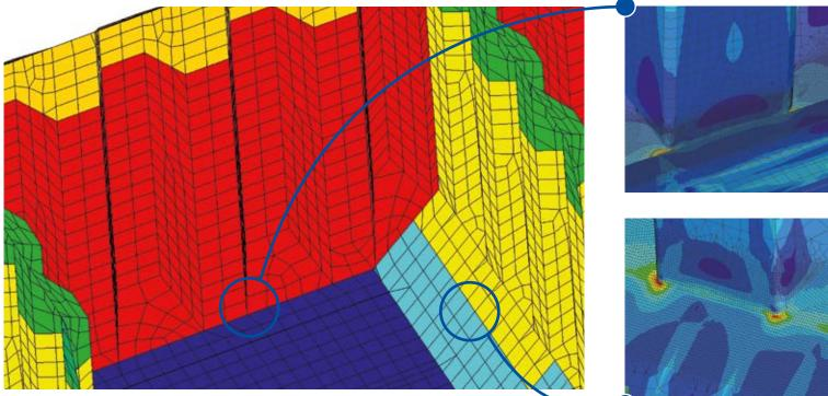
Feasibility study of product/chemical tanker. Cargo hold model with very fine mesh models of the hinges.
