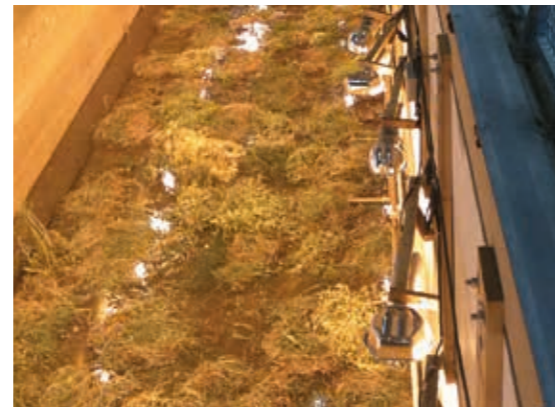
4.23 > Accurate measurements to determine how well a salt marsh with high-growth vegetation could reduce wave energy were made for the first time in a wave flume.
