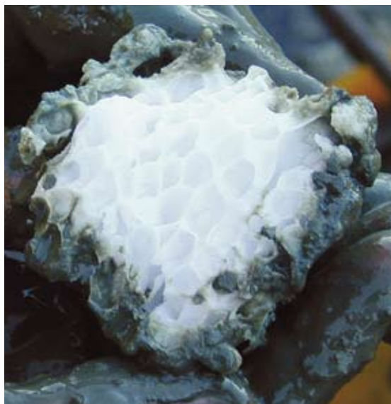
7.8 > Methane hydrates occur worldwide. This ice-like block with a honeycomb structure was obtained from the sea floor during a research expedition off the coast of Oregon.
