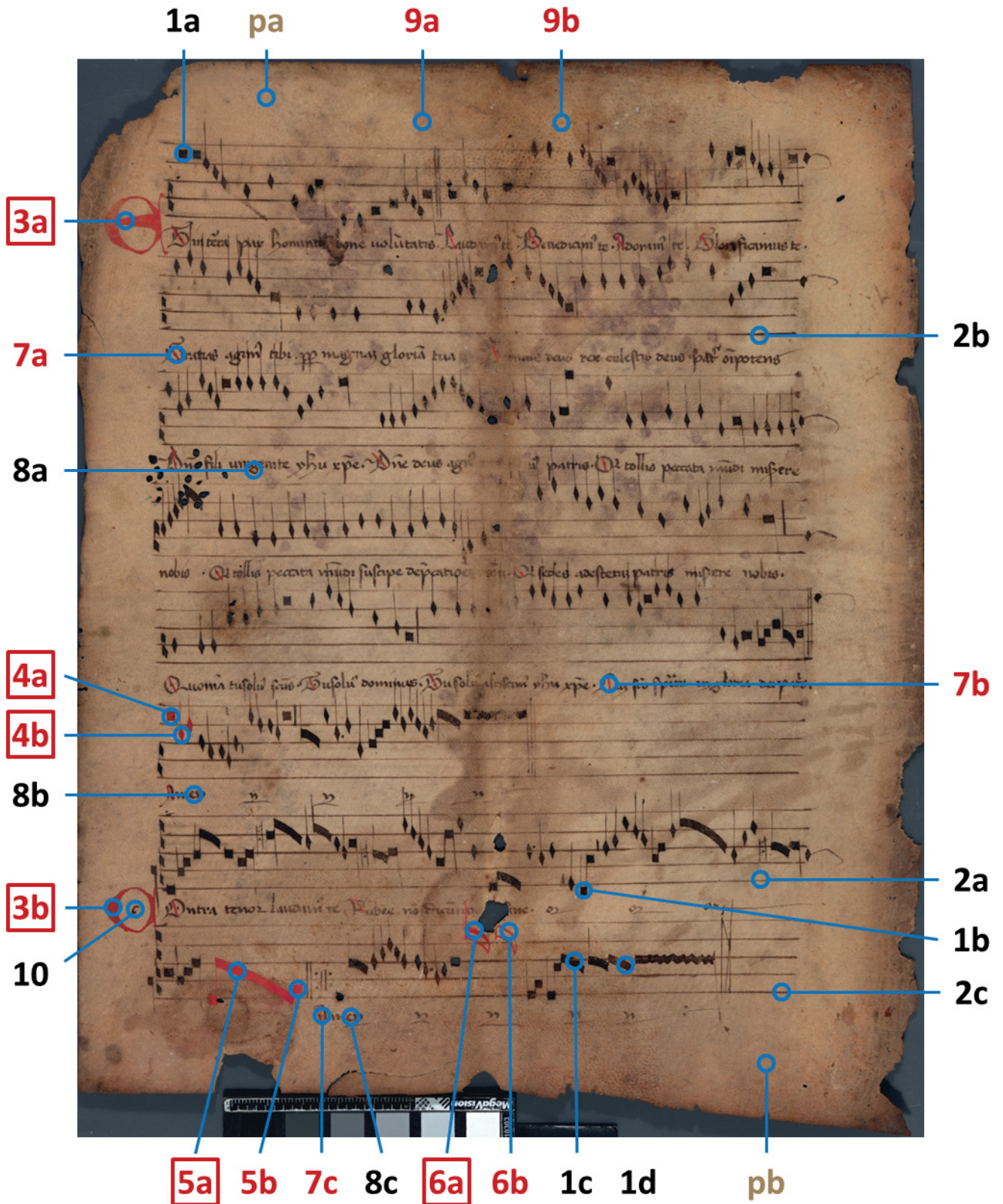
Fig. 5: Measured spots on the recto side of Atri Fragment . The black, brown and red numbering corresponds to XRF measurements. Numbers with a red frame indicate additional reflectance measurements by spectrophotometry.
