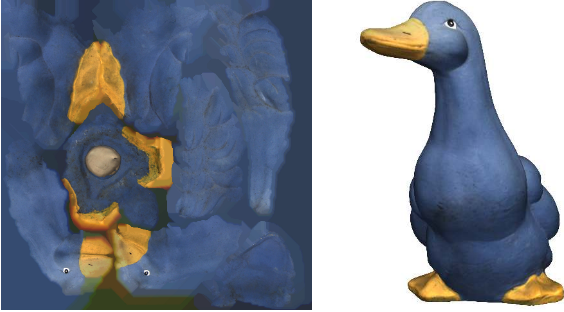
Figure 1. Left: Texture Bitmap as delivered by the scanner software. Right: Texture mapped onto the geometry.
