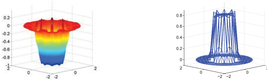
FIGURE 1. Control (left), and adjoint state (right) (variational discretization)
