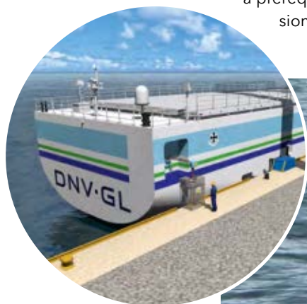
The DNV GL experimental-scale model ReVolt is used by NTNU in Trondheim to determine how advanced control systems and navigation software can control an unmanned vessel.
