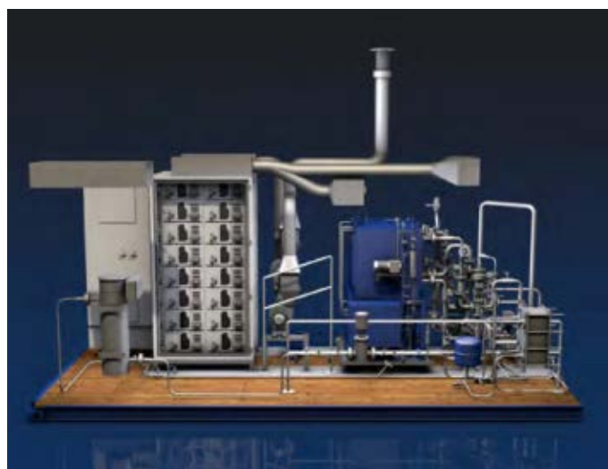
Project Pa-X-ell, one of the e4ships pilot projects, is putting high-temperature PEM fuel cells to the test on passenger vessels.
