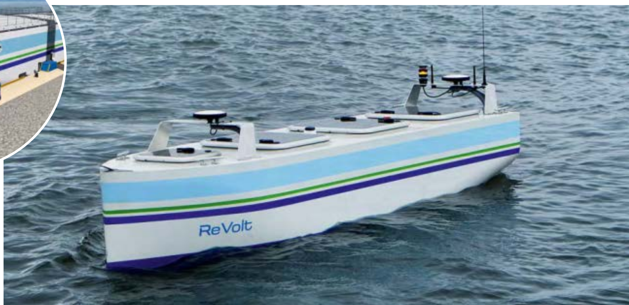
The DNV GL experimental-scale model ReVolt is used by NTNU in Trondheim to determine how advanced control systems and navigation software can control an unmanned vessel.
