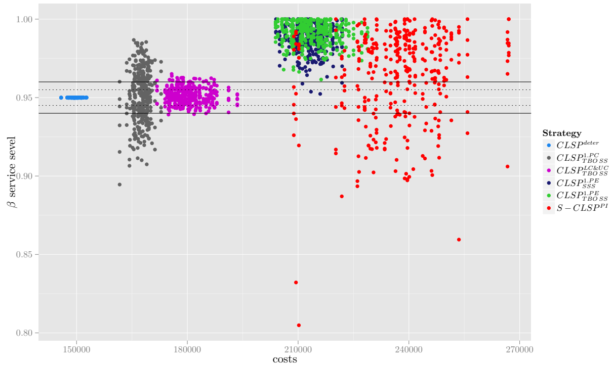
Figure 4 Trade-off between costs and \beta_j^{EI} service level for mixed TBO 's and a machine utilization of 85%
