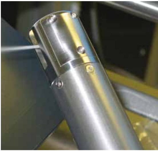
Figure 2 Lance with moveable nozzle. The nozzle can be moved steplessly from horizontal to vertical to realise various jet angles. It is used for 1.3 GHz RF guns with an iris diameter of 50 mm.
