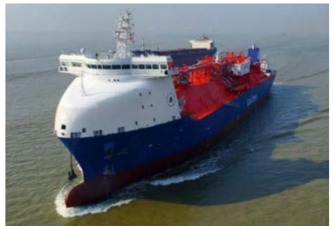
GasChem Beluga is the largest LEG carrier with Type-C tanks built to date.
