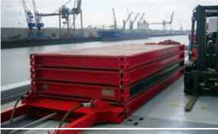
Lashing platforms carrying project cargo fall within the scope of CSC.
