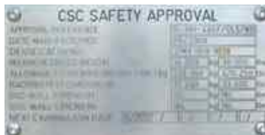
A valid CSC plate on containers and racks is mandatory.
