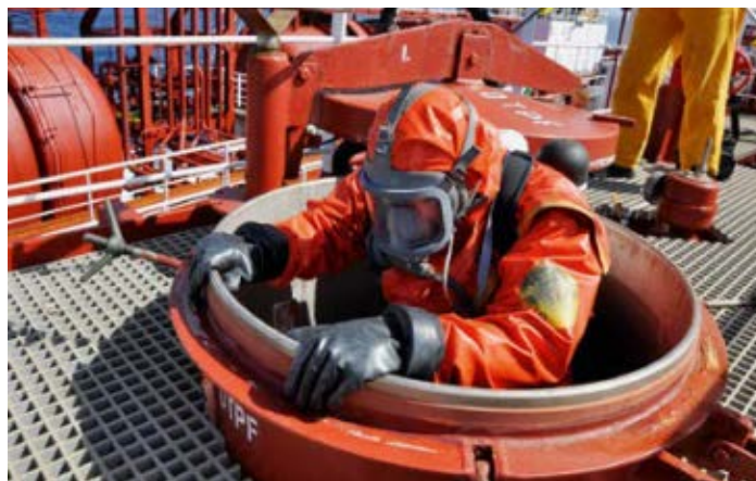
New safety requirements may call for breathing apparatus and protective gear for persons entering a tank that carried recategorized products.
