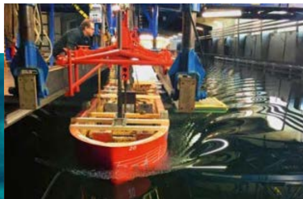
The traditional towing tank test confirms the improved propulsive efficiency.
