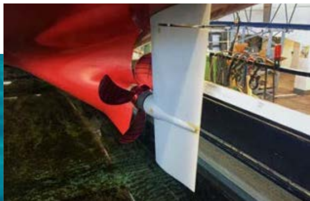
Tank test model of a handymax bulk asymmetric stern shape.
