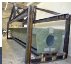
A full-size tween deck prototype was produced and tested and the design concept has received approval in principle (AiP) from DNV GL.
