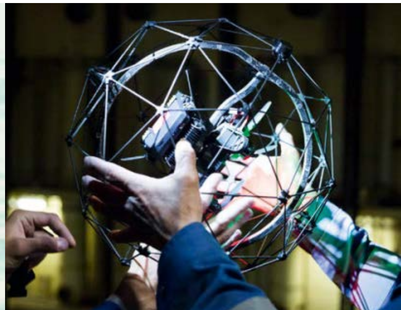
DNV GL surveyors perform a final check on one of the custom-built DNV GL drones, before using it to inspect a cargo tank.
