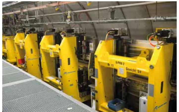
The sFLASH undulators in the FLASH tunnel.
