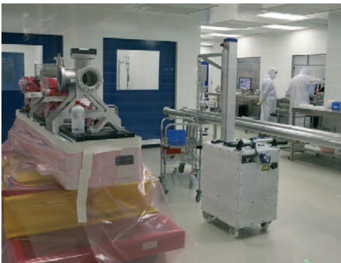
Figure 3 Installation of vacuum components on girders in the DESY cleanroom (August 2014)
