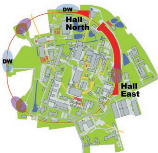
Figure 1 Overview of the PETRA III storage ring showing the new halls North and East. Each hall will house five beamlines.
