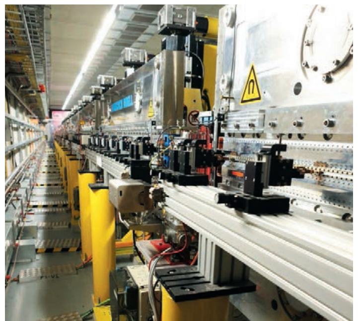
Undulator of FLASH2, the new beamline at DESY's FLASH free-electron laser facility
