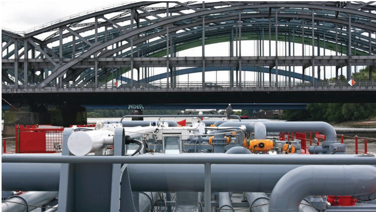
Passing safely under the Elbe bridges is a matter of centimetres. To avoid collisions, Mike has to lower the wheelhouse and the mast at the bow
