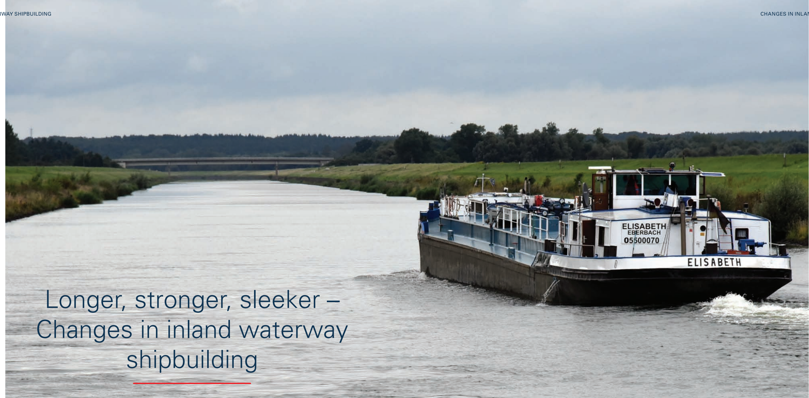
With locks and ship lifts just 12 metres wide, the Elbe Lateral Canal can only be used by inland craft with a maximum width of 11.45 metres
