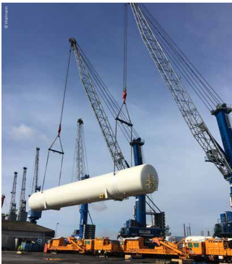
Strong performers: In twin operation Wallmann's mobile port cranes can hoist 400 tons
