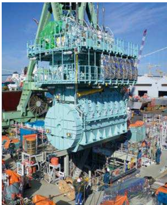
Lowering the gigantic dual-fuel engine designed by MAN Diesel & Turbo into the hull is high-precision work.
