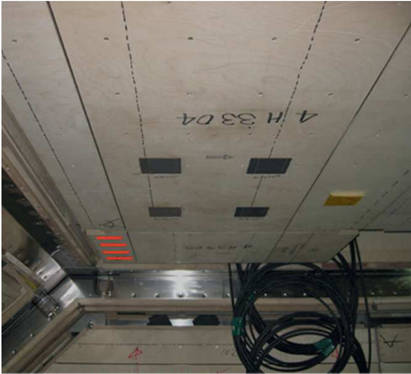
Fig. 1: Tank fully equipped with membrane. Insulation boxes fitted with pressure sensors and indication-of-strain gauges in a corner box
