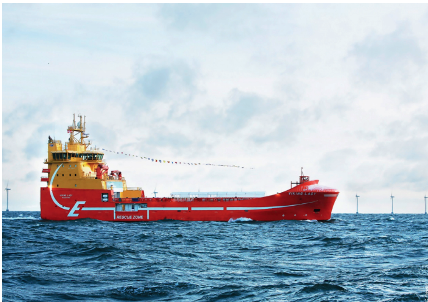
Figure 1. The Viking Lady OSV: the first full-scale hybrid-electric vessel.
