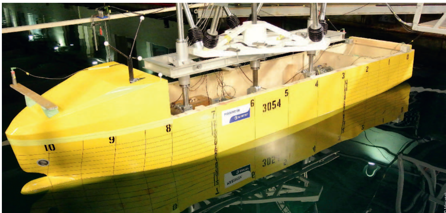
Setup for the forced roll motion model tests.
