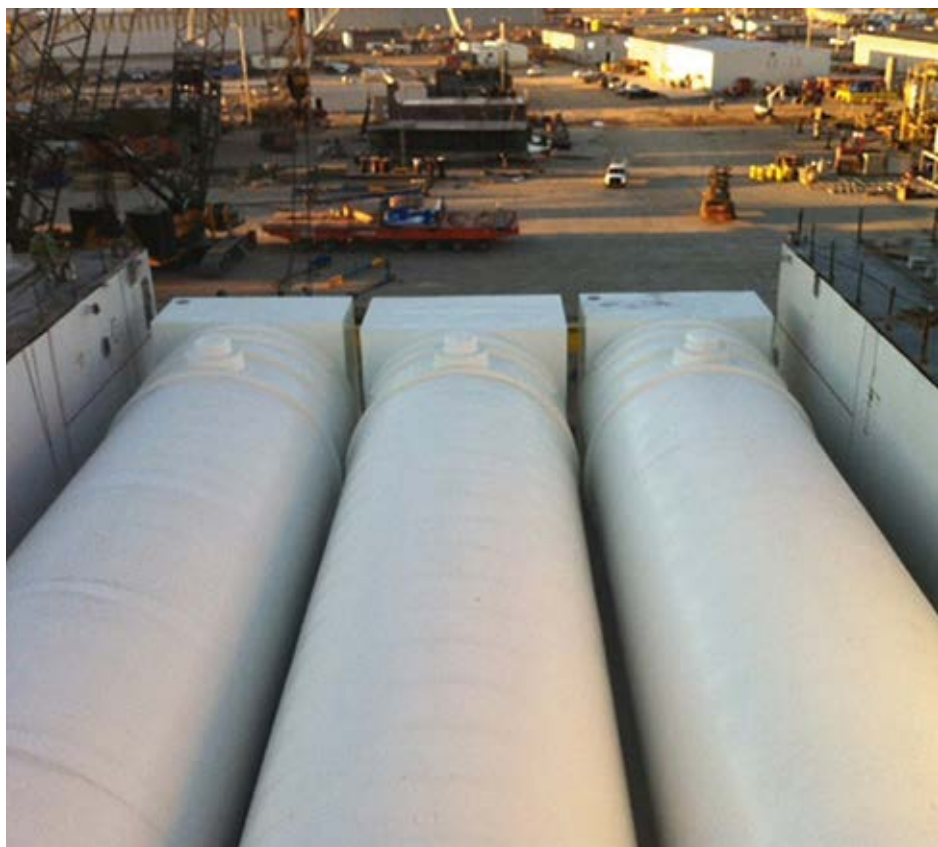
A TGE tank ready for shipment to NACKS for a PCTC ordered by United European Car Carriers (above left). Installation of three TGE LNG tanks on board a newbuild at shipyard VT Halter Marine (left and right).
