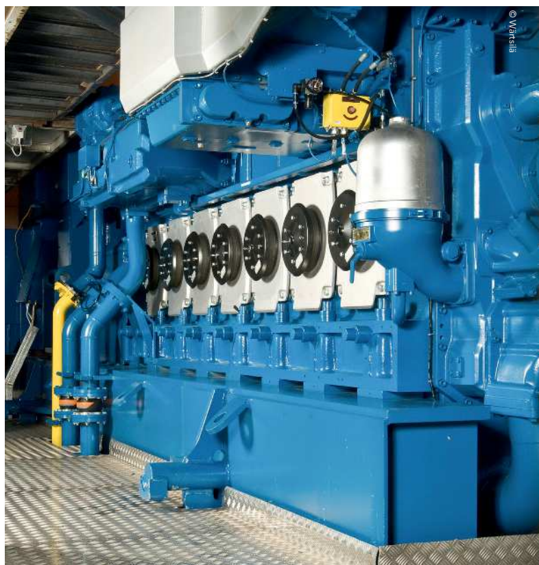
Wärtsilä 34DF, the midsize engine in the gas engine portfolio
