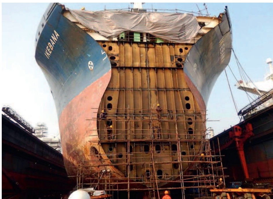
Preparing the IKEBANA for the fitting of the new bulbous bow at Chengxi Shipyard, China
