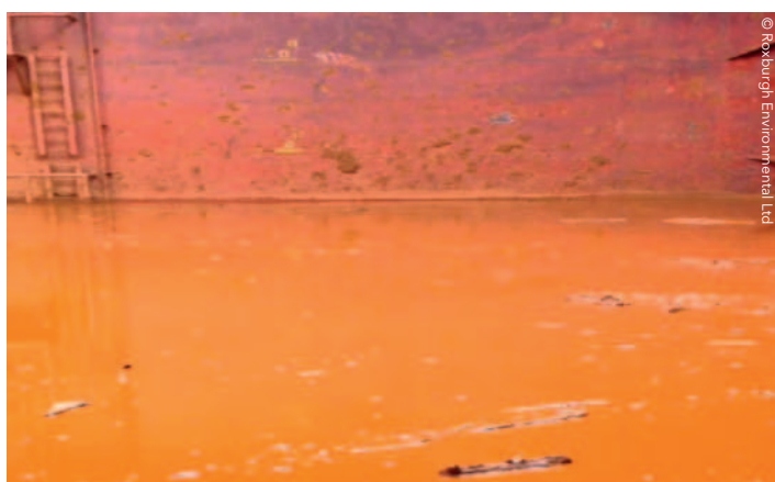
Cargo that has liquefied
