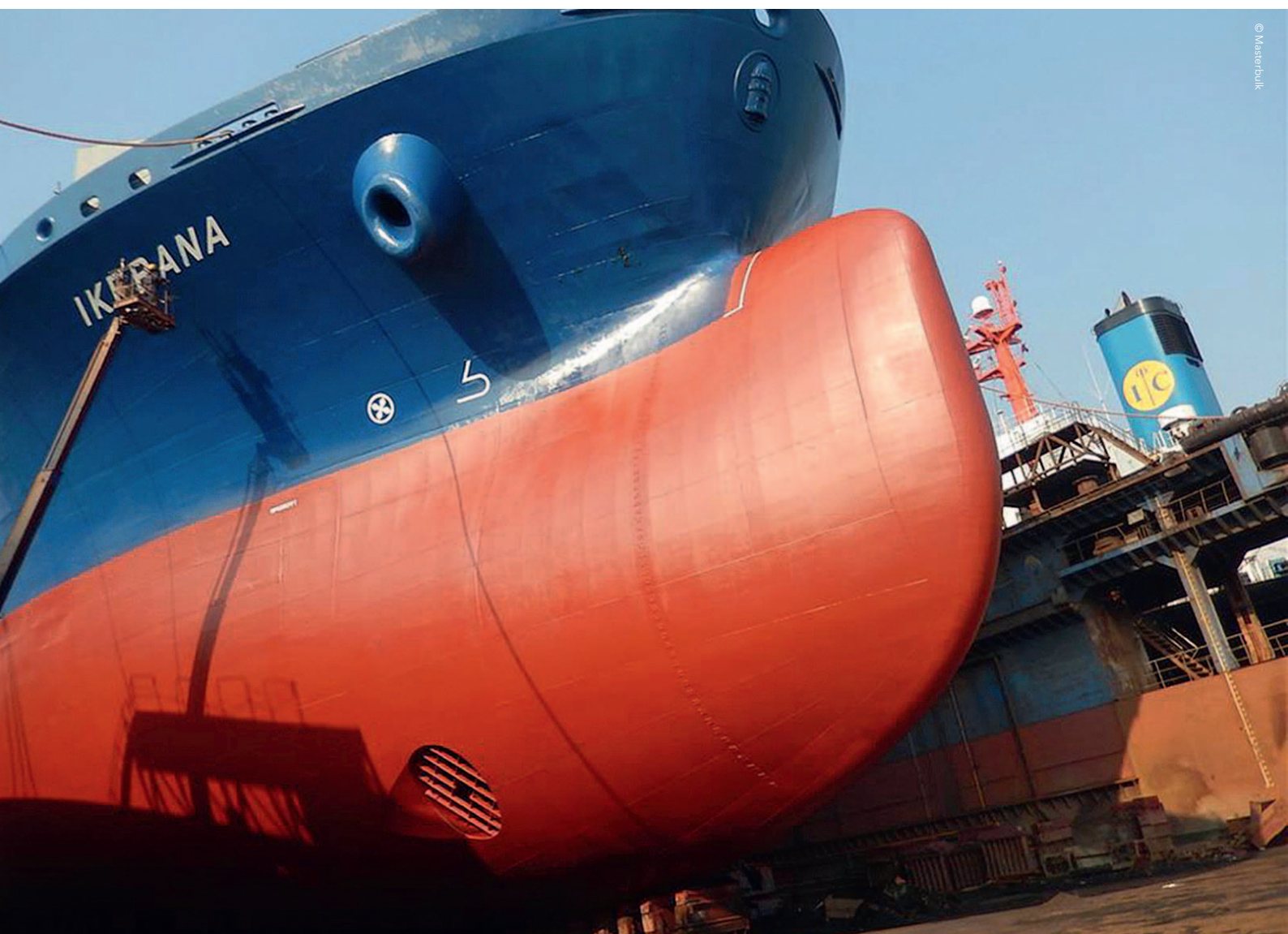
New bulbous bow fitted on the 45,000 dwt IKEBANA during drydocking at Chengxi Shipyard, China
