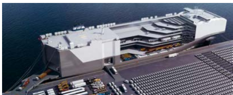
Höegh's record-setting, 200-metre PCTCs will each carry up to 8,500 vehicles on 14 cargo decks.
