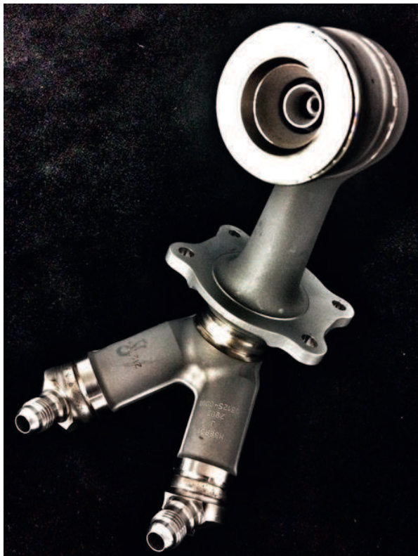
Figure 7. Examples of using the direct energy deposition process for part repair. (I. Gibson, D. W. Rosen and B. Stucker, ed., Additive Manufacturing Technologies: Rapid Prototyping to Direct Digital Manufacturing, Springer, 2010.).
