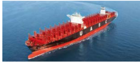
Sajir , the first LNG-ready ultra-large container vessel, set a precedent for the use of alternative fuels in the 15,000 TEU segment.
