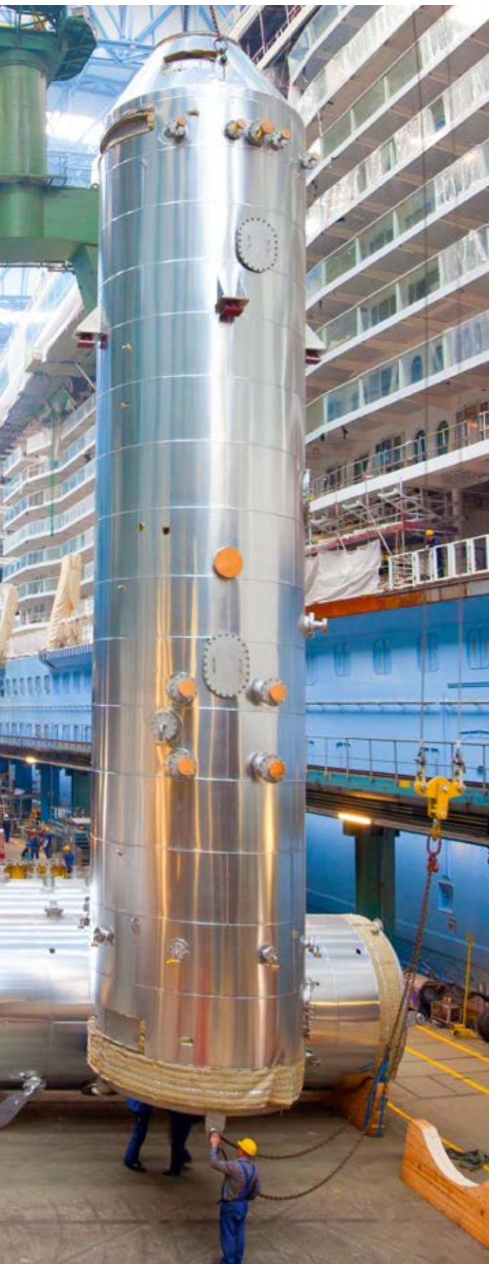
Scrubbers ready for installation on board Norwegian Escape at Meyer Werft. These are the biggest inline scrubbers worldwide.
