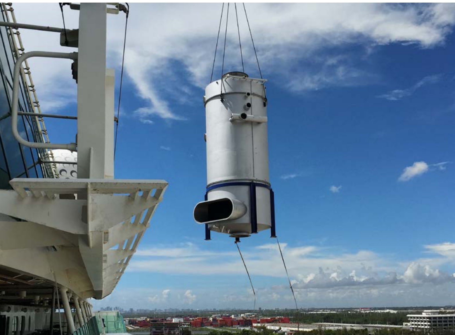
A scrubber being hoisted onto a cruise vessel owned by Royal Caribbean Cruises.
