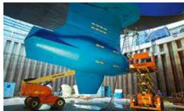
The Azipod propulsion system cuts fuel consumption and emissions to air.
