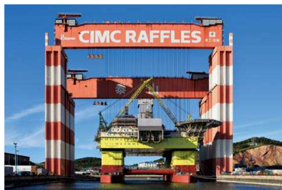
COSL Prospector, sitting under CIMC’s 20,000-tonne “Taisun” crane after the completed mating procedure.
