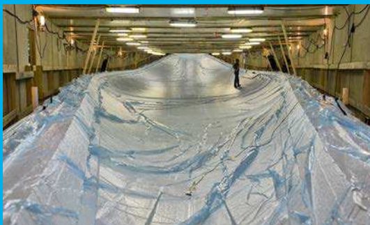
The SPRINT vacuum process ensures resin saturation.
