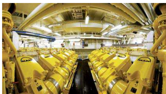
Modern ship engines replace the camshaft with an electronic valve control system.
