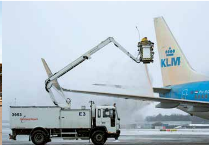
In winter, aircraft de-icing operations, made necessary by weather conditions, can lead to pollution of surface water
