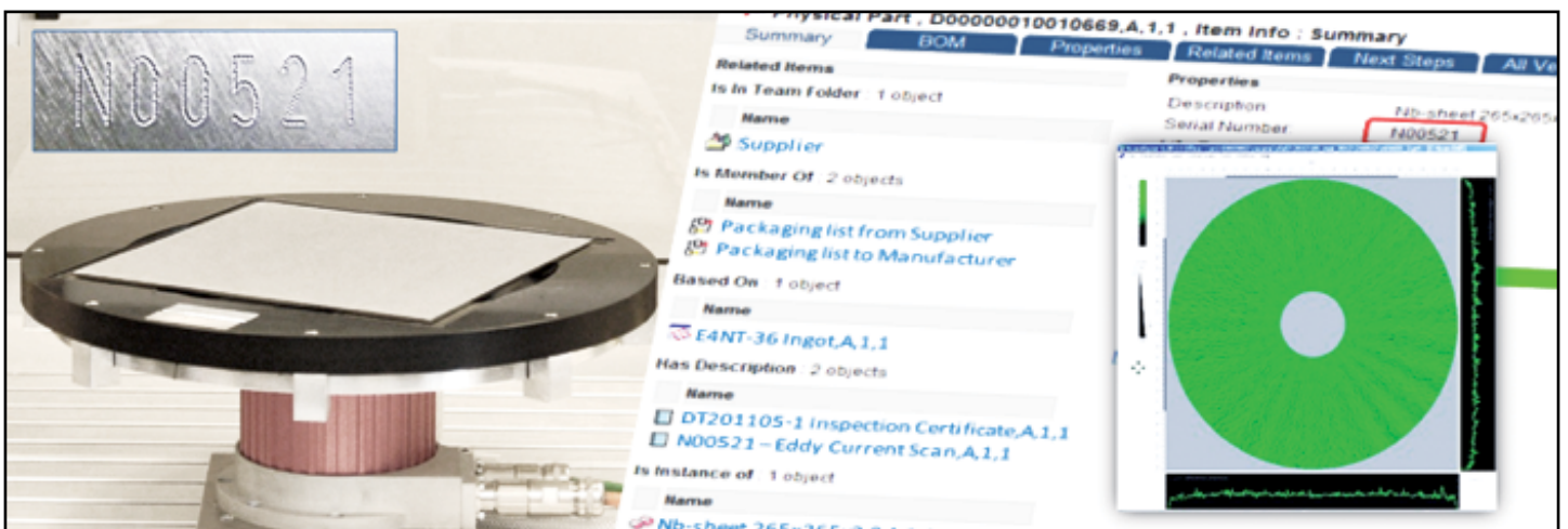
Figure 2 Example of a niobium sheet that was used in the production of a superconducting RF cavity: the sheet has a tracking number (left), the EDMS contains all supplier, shipment and inspection records, and tracks where and when the sheet has been used (right).
