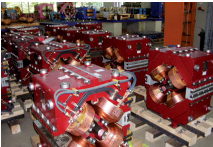
Quadrupole magnets for the extension of the PETRA III synchrotron radiation facility
