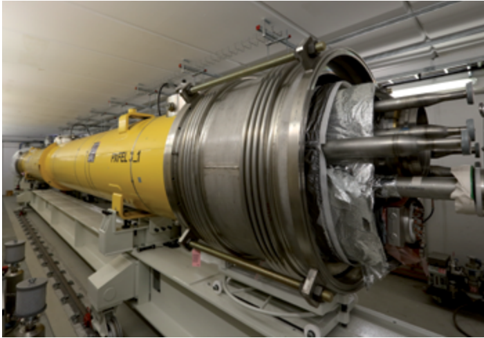
Superconducting accelerator modules for the European XFEL X-ray laser are being measured on test benches in DESY's Accelerator Module Test Facility (AMTF).
