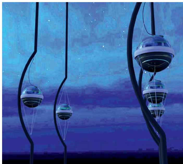
Impression of IceCube's digital optical modules, arranged in strings
