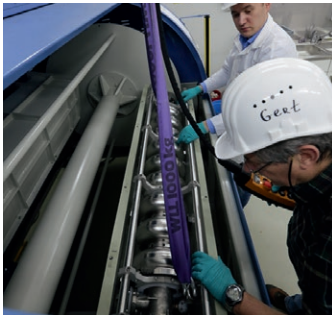
Figure 3 Cavity being lowered into the housing of the polishing apparatus
