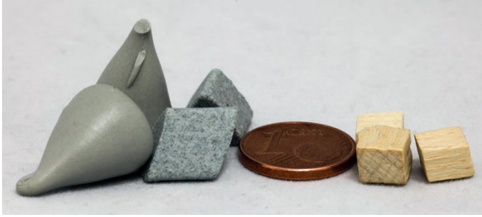
Figure 2 Abrasive materials used for "stone washing" the cavities
