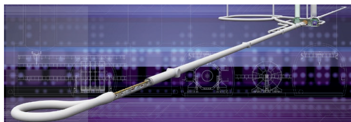
The two linear accelerators at the heart of the ILC will be built using the superconducting TESLA technology originally developed at DESY.
