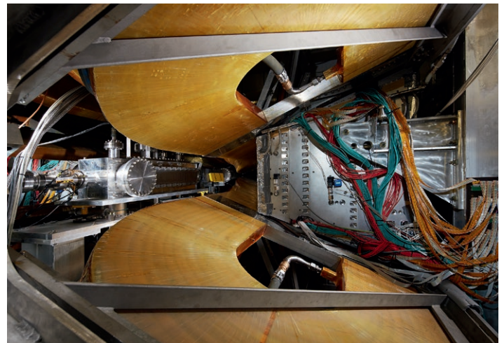
Figure 2 Picture of the OLYMPUS detector, showing the target chamber in the beamline, one of the drift chambers and part of the toroidal magnet
