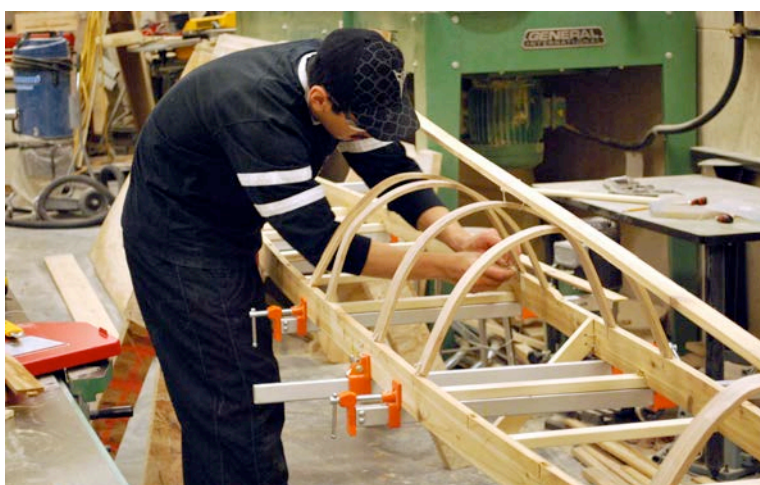
Figure 28. A student binds steamed kayak ribs with caribou sinew in the high school carpentry shop.
