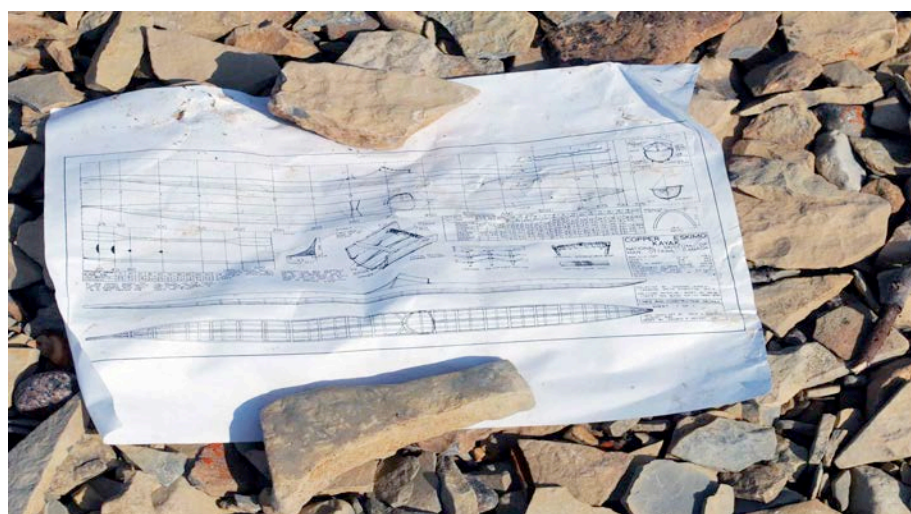
Plate 9: Line measurements taken from a Copper Inuit kayak (CMC IV-D-1057) housed at the Canadian Museum of Civilization (Zimmerly 1985:10). On the first day of our kayak building workshop in Cambridge Bay (see below), I provided this line-drawing as a map to guide measurements for reconstruction of the boat. The map was discretely placed on the ground, where it remain unused until the project was over.
