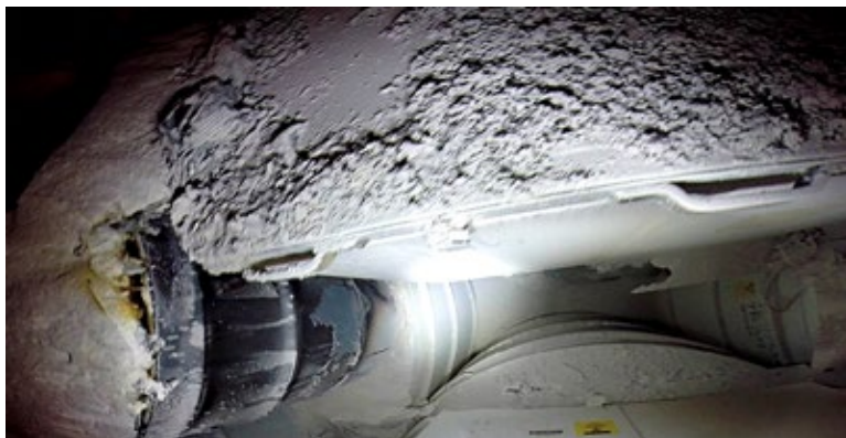
A damaged nuclear-waste container at Los Alamos National Laboratory, with its lid unsealed and apparent heat discoloration in evidence
