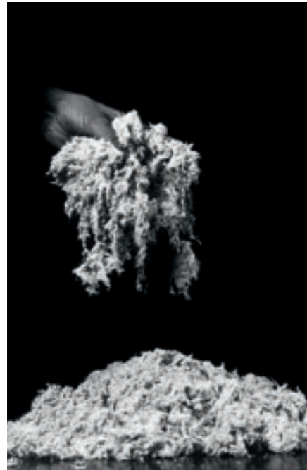
Left: Quality control of the 'miracle fibre' as asbestos was once called because of its resilience, resistance to heat and acidity and its good insulating properties.
