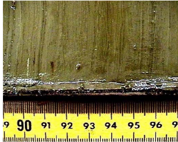
Fig. 46 Color photograph showing exposed varved structure of a piston core from the Santa Barbara Basin. This particular sediment is about 250 years old, with increasing age from left to right. Each varve is composed of one dark/light couplet. Scale is in cm. From http://php.indiana.edu/~aschimme/ .
