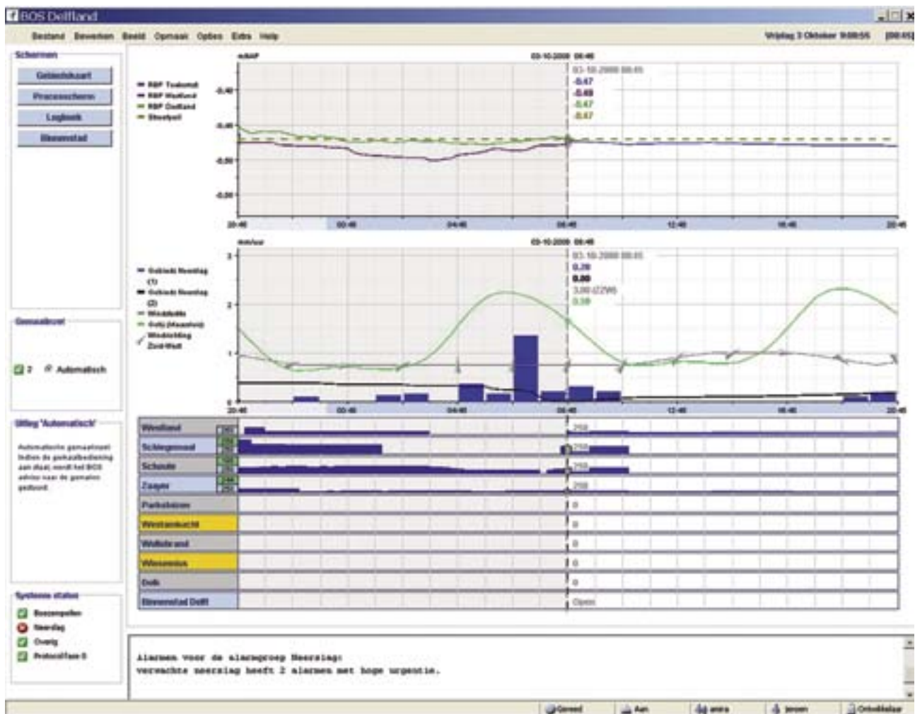
Figuur 1 BOS Delfland. Used for everyday automatic control of main pumping stations
