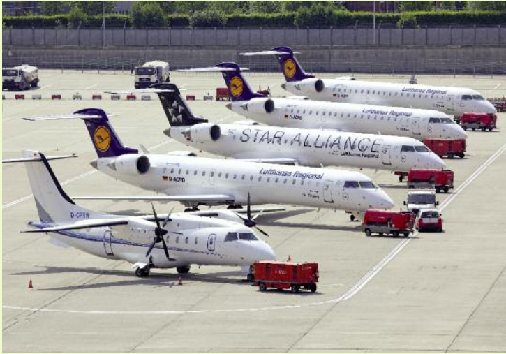
Diesel generators (Ground Power Units) supply electricity to aircraft at remote positions.
