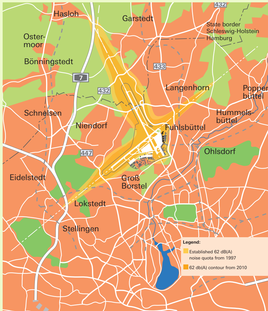
Prescribed noise quota from 1997 (area: 20.39 km 2 ) and development of noise levels by 2010 (13.34 km 2 ).
