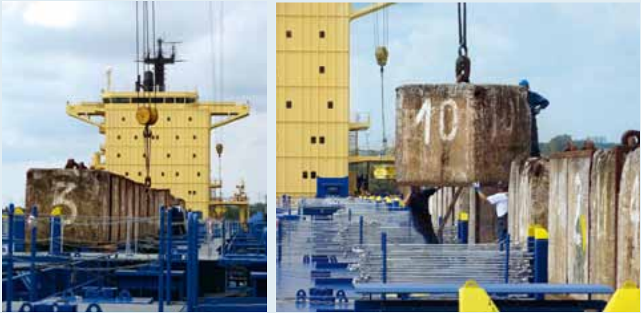
ARRANGEMENT. During an inclining test, known weights produce a heeling moment for measuring the change in the equilibrium heel angle.
