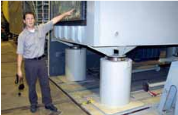
TEST. GL expert Dr Christof Weibenborn at the window test stand, which emulates the acoustic characteristics of ship structures. The surface velocity of the glass pane under test is measured by means of a scanning laser vibrometer.
