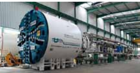
GIGANTIC. The shield tunnelling machine for Hamburg's new underground line U4.
