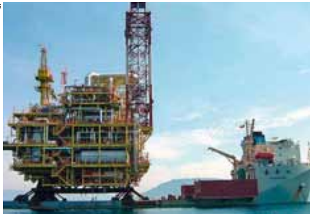
TRANSPORT. A Talisman topside being transported to its destination, the PM-3 project between Malaysia and Vietnam.
