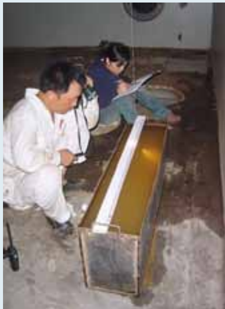
TEST. The heeling angles of a vessel in light-ship state are measured using leads.
