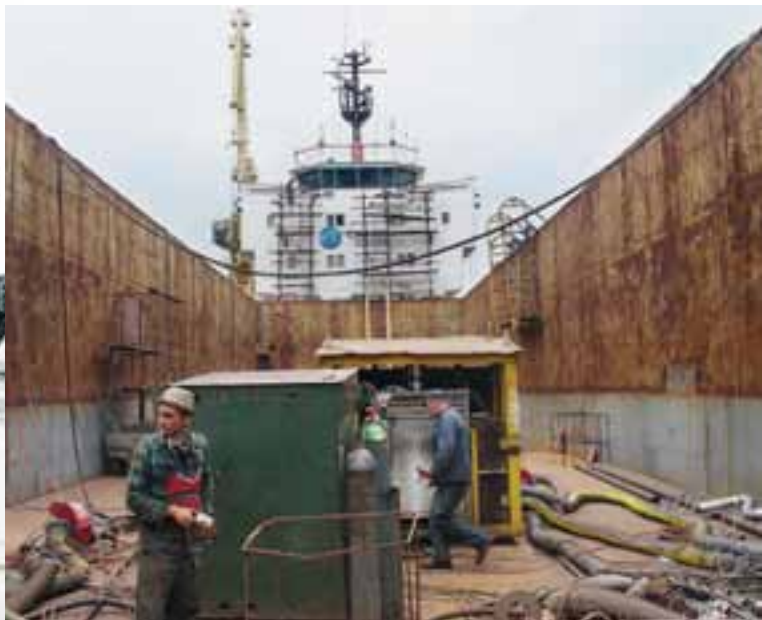
STRUCTURE. At the Remontowa shipyard in Szczecin, workers subdivided the hull lengthwise into chambers. When under way, these cavities will be filled with air from large compressors.
