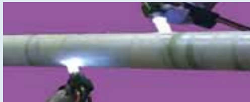
FIGURE 9. Flame spray application of PP.
